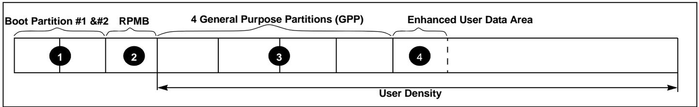
Figure 6. Example of Partition Configuration
